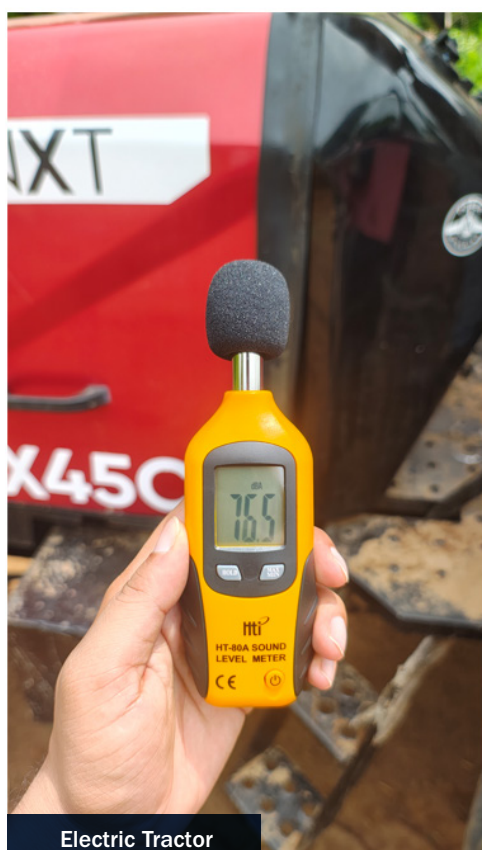
Figure 13: Comparison of Sound Pressure Level from Electric and Diesel Tractor
