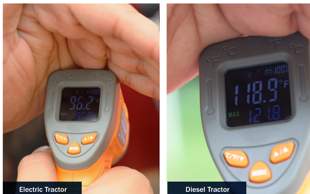
Figure 14: Comparison of Temperature Around the Operator's Seat in Electric and Diesel Tractor
